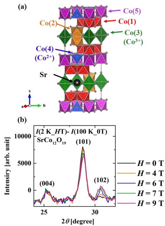
Fig. 1. (a) Crystal structure of SrCo<sub>12</sub>O<sub>19</sub>. (b) Neutron diffraction profiles at 2 K under several magnetic fields. The profile at 100 K under zero field is subtracted from the profiles as the background intensities.
